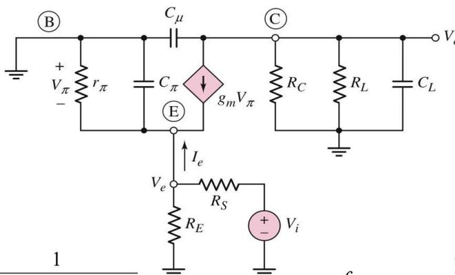
$$f_{H\pi} = \frac{1}{2\pi \left[ \frac{r_{\pi}}{1+\beta} \parallel R_B \parallel R_S \right] C_{\pi}}$$
