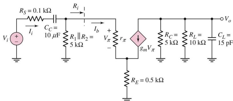
$$f_L = \frac{1}{2\pi[R_S + (R_1 \parallel R_2 \parallel R_i)]C_C} \quad (b)$$
