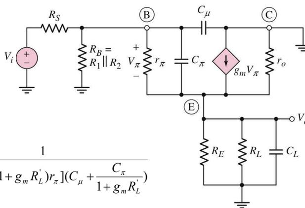
$$f_H \cong \frac{1}{2\pi[R_S \parallel R_B \parallel (1 + g_m R'_L)r_\pi](C_\mu + \frac{C_\pi}{1 + g_m R'_L})}$$
