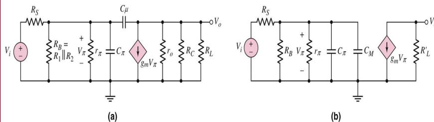
$$f_H = \frac{1}{2\pi[r_\pi \parallel R_B \parallel R_S](C_\pi + C_\mu)}$$
