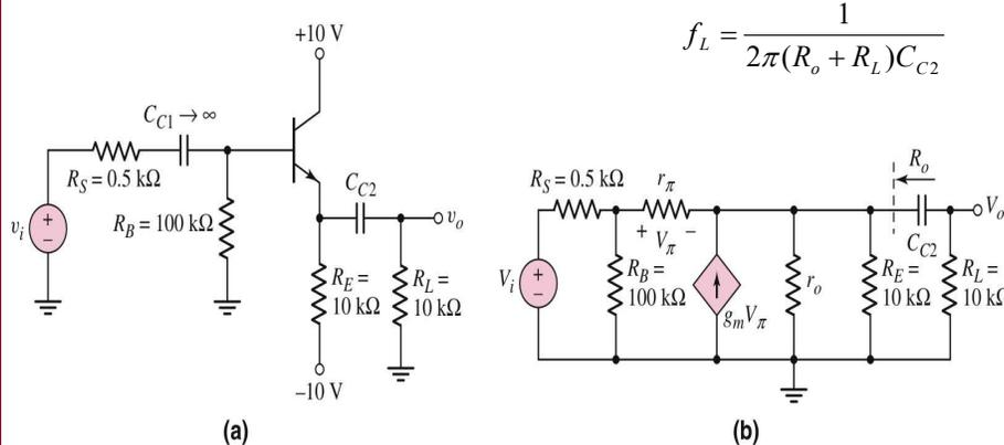
$$f_L = \frac{1}{2\pi(R_o + R_L)C_{C2}}$$
