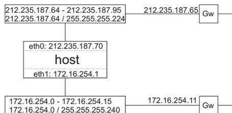
Figure 2.10: Host connected to two subnets with two network interfaces
