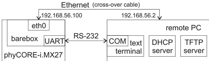
Figure 4.2: phyCORE-i.MX27 embedded system connection to a remote PC
