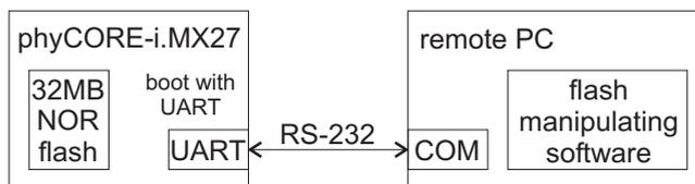
Figure 4.1: Erasing the NOR flash and uploading a boot-loader
