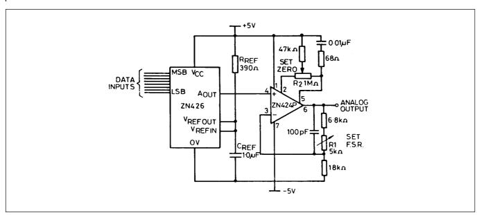
Fig.4 8-bit D-A converter
