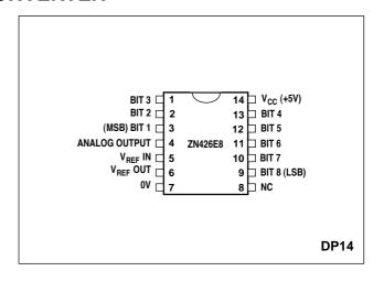
Fig.1 Pin connections (not to scale) - top view
