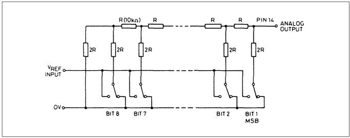
Fig.3 The R-2R ladder network
