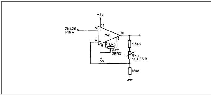
Fig.5 The ZLD741 as output buffer
