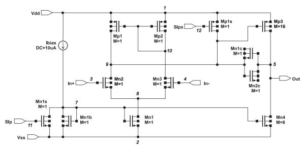
Fig. 8 A simple operational amplifer.
