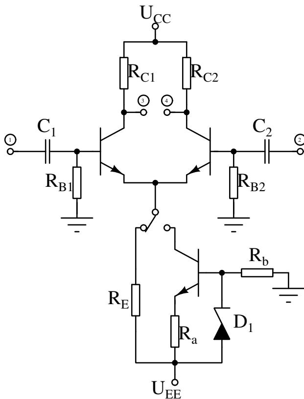
$$\begin{aligned} U_{CC} &= 10V, U_{EE} = -10V, \\ R_{C1} &= 3.9k\Omega, R_{C2} = 3.9k\Omega, \\ R_{B1} &= 180k\Omega, R_{B2} = 180k\Omega, \\ R_E &= 3.9k\Omega, \\ C_1 &= 1\mu F, C_2 = 1\mu F, \\ U_{D1} &= 4.7V \text{ pri } I_{D1} > 5mA, \\ R_a &= 1.5k\Omega, R_b = 470\Omega \end{aligned}$$
