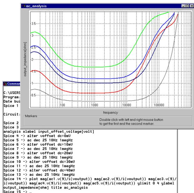
Figure 3: The output impedance at different biases
