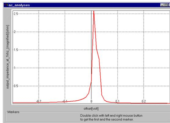
Figure 5: The output impedance vs. the input offset
