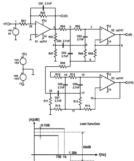
Figure 1: Active low-pass RC filter
