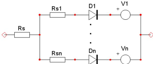
Figure 2: Zener diode differential resistance model.
